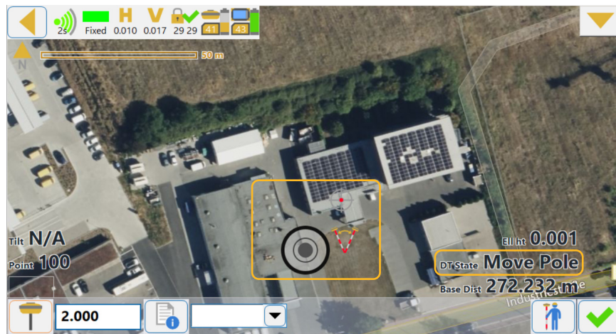
Figure 3-13: TILT Move Pole State
