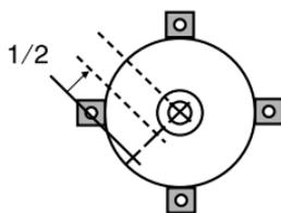
5. Use the 4 adjusting screws of the optical plummet to adjust the remaining half of the deviation as shown below.
