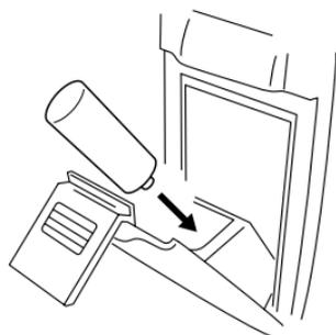
Firmly insert the batteries after verifying the direction in which they go.
