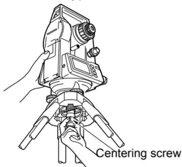
3. Looking through the optical plummet eyepiece screw, turn the optical plummet eyepiece to focus on the reticle. Turn the optical plummet focusing ring to focus on the survey point.
