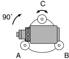
5. Turn the upper part of the instrument a further  $90^\circ$  and check to see if the bubble is still in the center of the plate level. If the bubble is off-center, perform the following:
